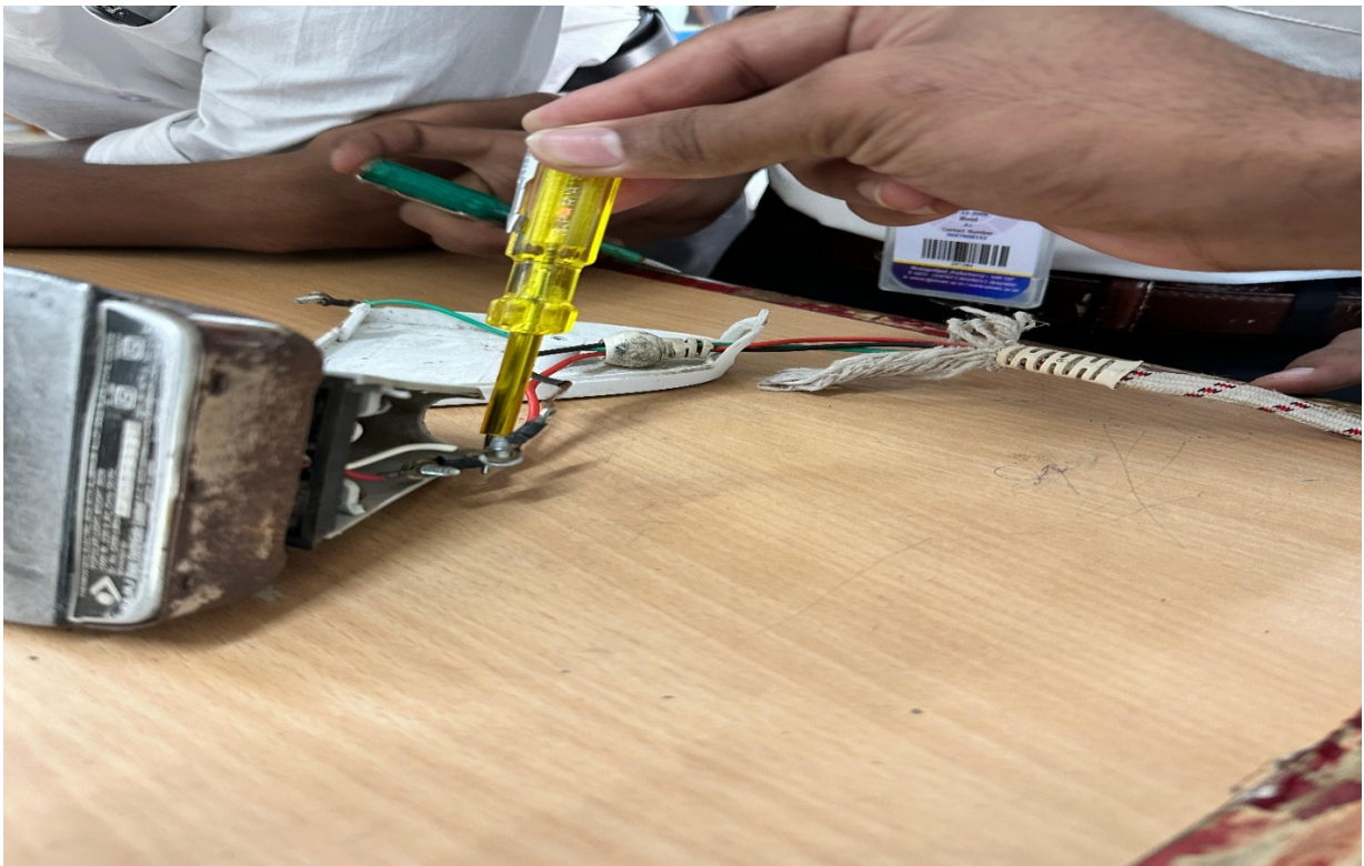
After rectifying the iron box, the students verify the power supply using an electrical tester to ensure proper voltage and secure connections
