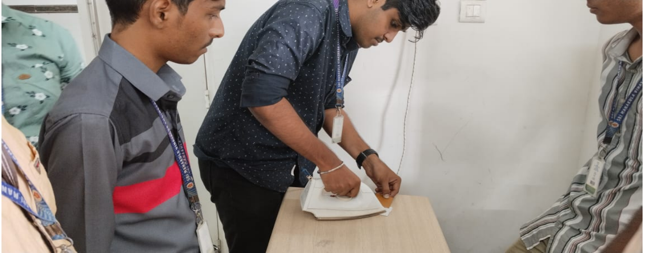
Students are transferring the Marker's Ink layout to the top of Copper Plate.
