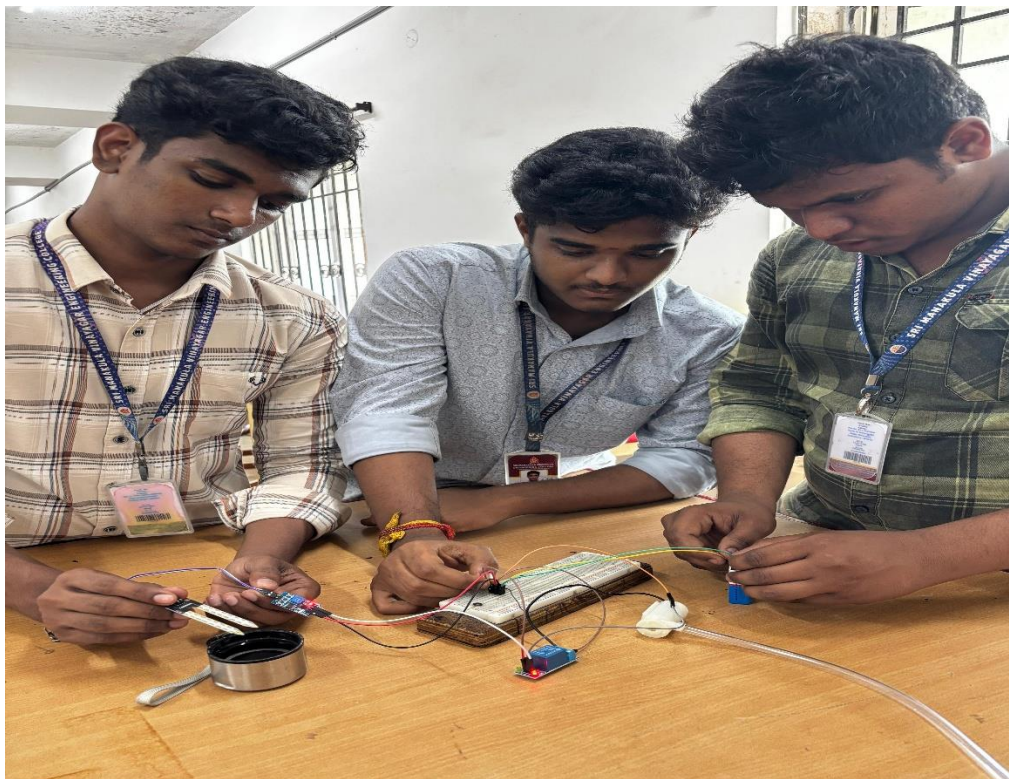
The students are engaged in the practical implementation of the Automatic Plant Watering System prototype, involving the connection of the moisture sensor, control circuit, and water pump for testing purposes.
