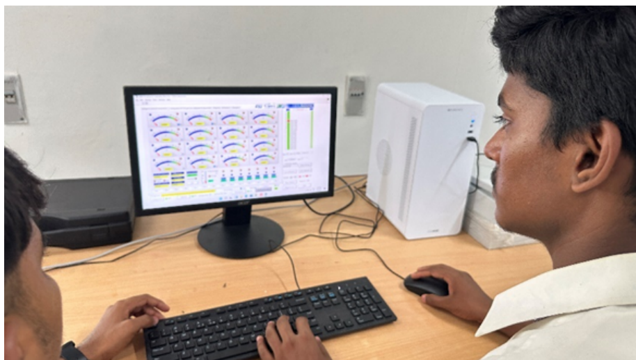
BMS continuously monitors battery voltage, current, and temperature to ensure safe operation
